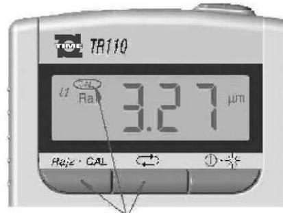
Press the Start Key to exit the status of Calibration. After calibration, the calibrated measuring value Ra will show on the screen. (At the meantime, the new standard sample plate value Ra will be stored to the memory instead of the old one). After the sensor returns to its original place, the tester can be used to make normal measurement.
