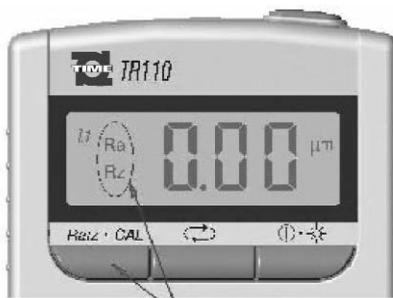
Picture 4 Ra/Rz conversion by press the left key gently and quickly
