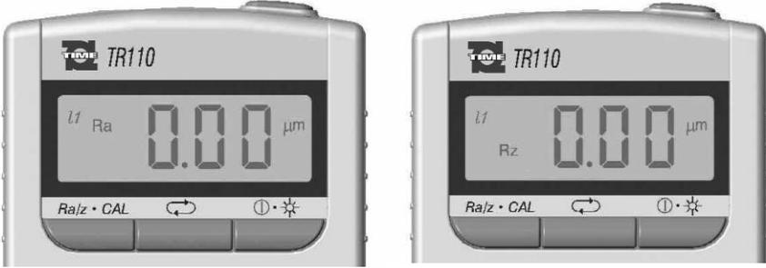
Press the Middle Key gently and quickly to select the sampling length (0.25mm, 0.8mm, 2.5mm) by turns. (Refer to Picture 5)
