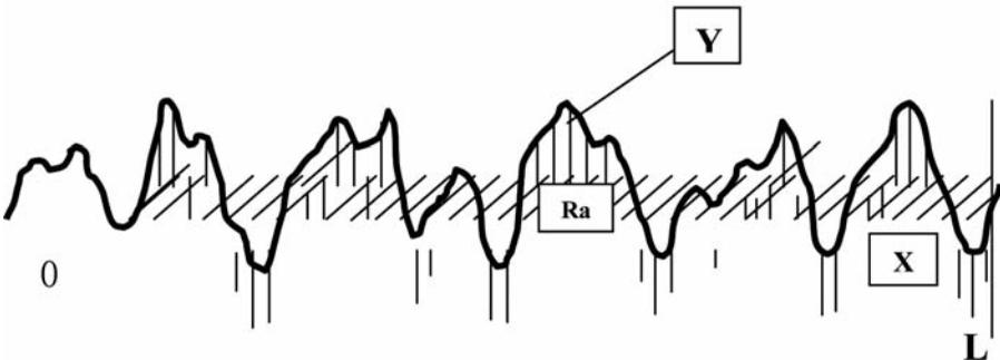
**Rq:** Root-mean-square Deviation of Profile is the root-mean-square of the deviation of profile within sampling length.
