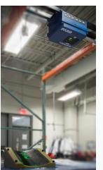
Both Laser Projectors, when paired with BuildIT Projector Software that has the new ScanAlign feature, can be used to automate alignment with retro-targets.
