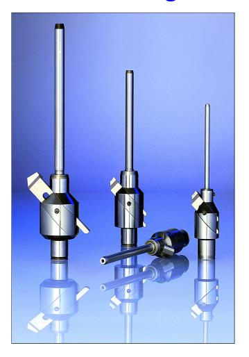
The VGX-21 tooling system features unique and exchangeable DT-Toolheads for the rapid and easy adjustability to the desired seat dimensions.
