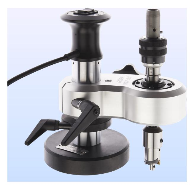
The portable VGX-21 valve seat refacing unit has been developed for the specialised petrol and diesel cylinderhead workshop. The highly accurate valve seat processing is achieved by a spherical spindle guide bearing as well as a unique hydraulic ball clamping system. A almost pressure free centering and braceless fixing of the MIRA rotary head is made possible in order to achieve precise and concentric valve seats! Order Number: VGX-21
