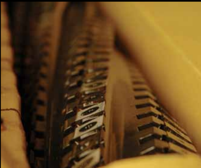
HELICAL CUTTERHEAD True helical cutterhead with 174 individual cutters.
