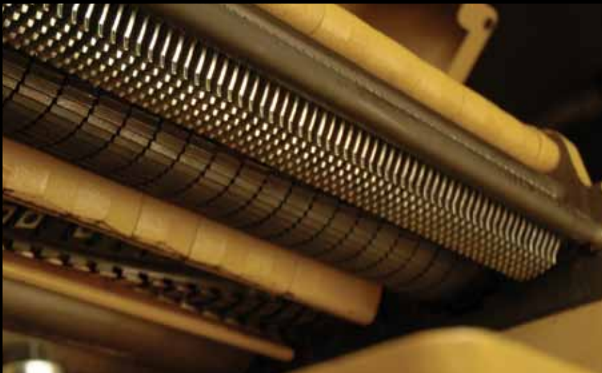
PLANER ASSEMBLY Segmented and serrated steel infeed roller for kickback protection.
